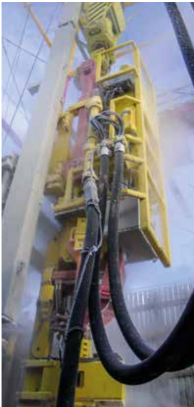
Portable Rotated Design (Dual Rail) The preferred solution to eliminate modifications on older mast designs capable of Top Drive operations.
