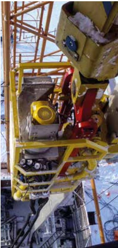
Portable Rotated Design (Mono Rail) The configuration of choice to avoid any mast modification on existing and narrow mast designs.
