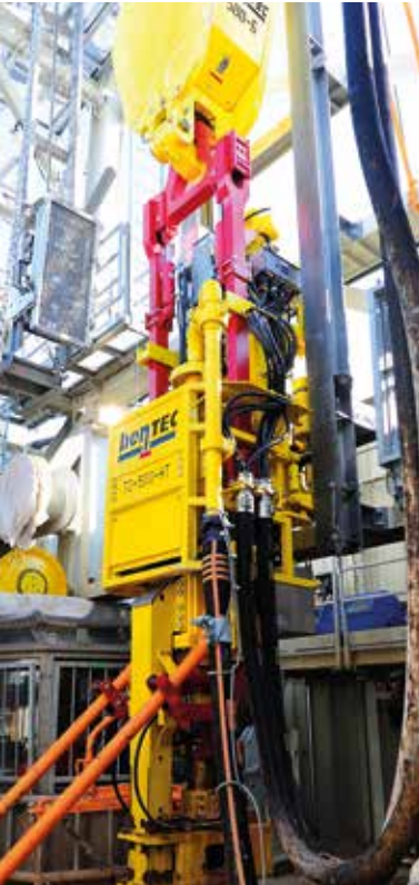
Integrated Rail Design Top Drive guide rails are an integrated part of the mast structure eliminating lifts and transport during rig move.
