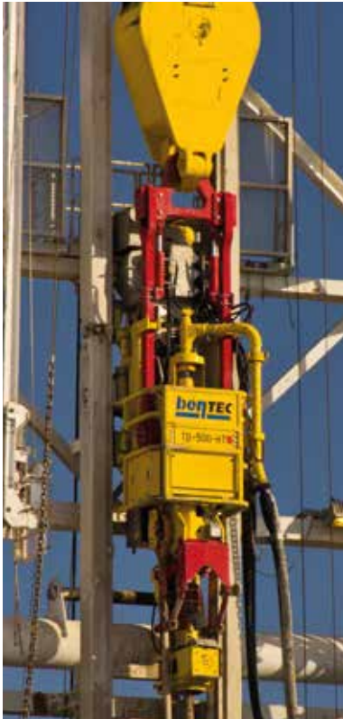
Portable Design Hanged-off portable rails in the mast with a torque reaction beam on the lower mast section enables high flexibility and usage over multiple rigs.
