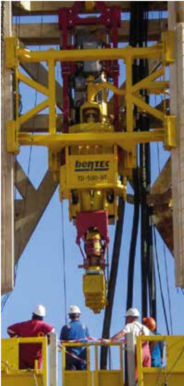
Herringbone Design The Top Drive carriage runs between the masts front legs, optimising rig moves by reducing lifts and rig move loads, to a minimum.
