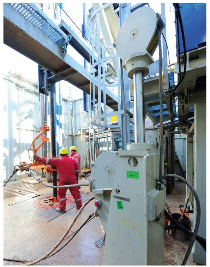
This useful rig floor equipment provides smooth and adjustable make-up Torque. Due to its hydraulic operation, the Bentec Hydraulic Cathead eliminates electrical hazards. The system can be powered by either a stand-alone hydraulic power unit (HPU), or integrated into the existing rig hydraulic power unit.
