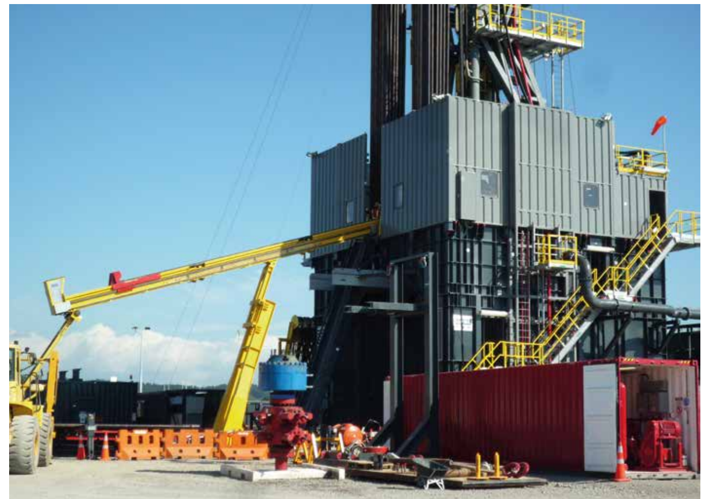
Special Design: Noise reduced Catwalk System with lowest possible elevation.
