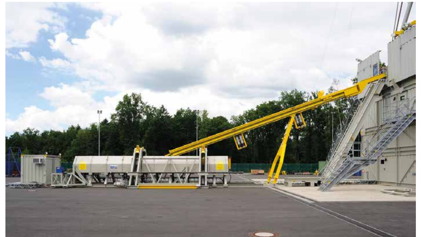
Special Design: Mechanized Catwalk System with elevation to work above wellheads.
