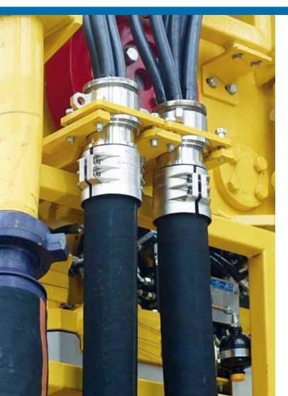
Bentec SERVICE LOOPS provide a highly reliable power and control supply solution for all common Top Drives and are interchangeable with the OEM service loops. By casting the power plugs and the end of the outer tubes, Bentec SERVICE LOOPS are able to withstand harsh environments and highest mechanical tractive forces.
