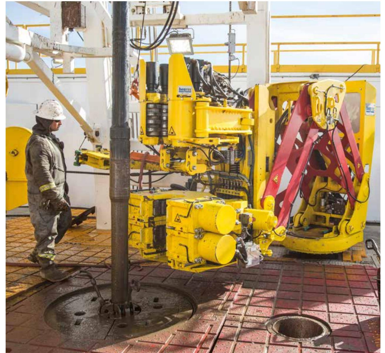
The Bentec Iron Roughneck provides a safe and versatile alternative to conventional pipe connection techniques for make and break operations.
