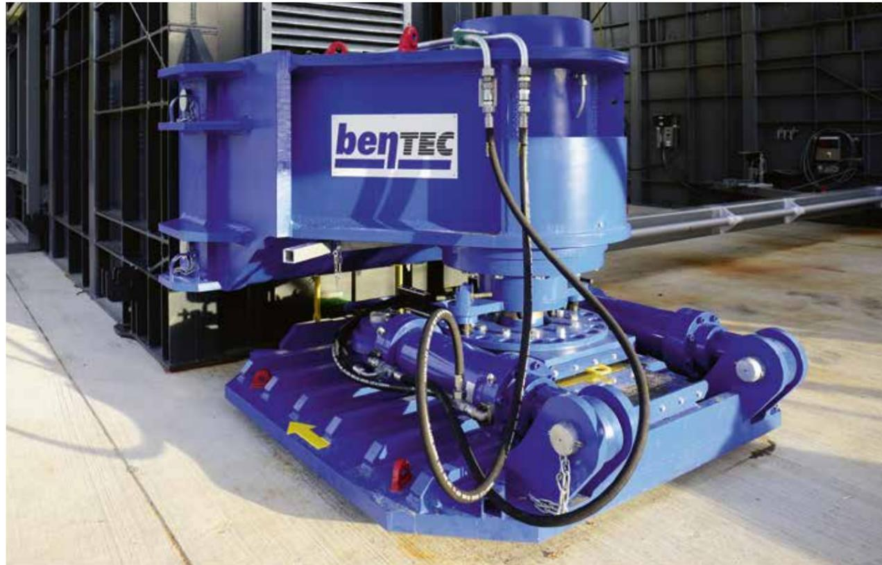
Bentec Rig Walking Systems provides a solution for reducing the time taken for a rig move on multi-well rig-sites. Moving the complete rig to the next well also requires fewer cranes and less manpower.
