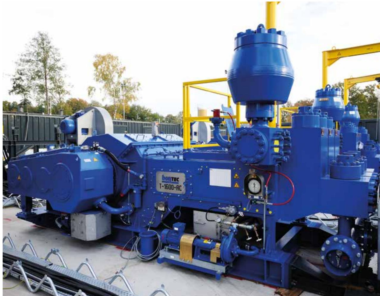
Bentec have completely redeveloped the concept of Mud Pumps. Equipping our Mud Pumps with a direct drive gearbox, Bentec AC-Motor and a state of the art pump housing. There is no requirement for an internal gear, with its many disadvantages and no more belt/chain tensioning. Bentec Mud Pumps are constructed to do the task that they are intended for: *pumping operations*.
