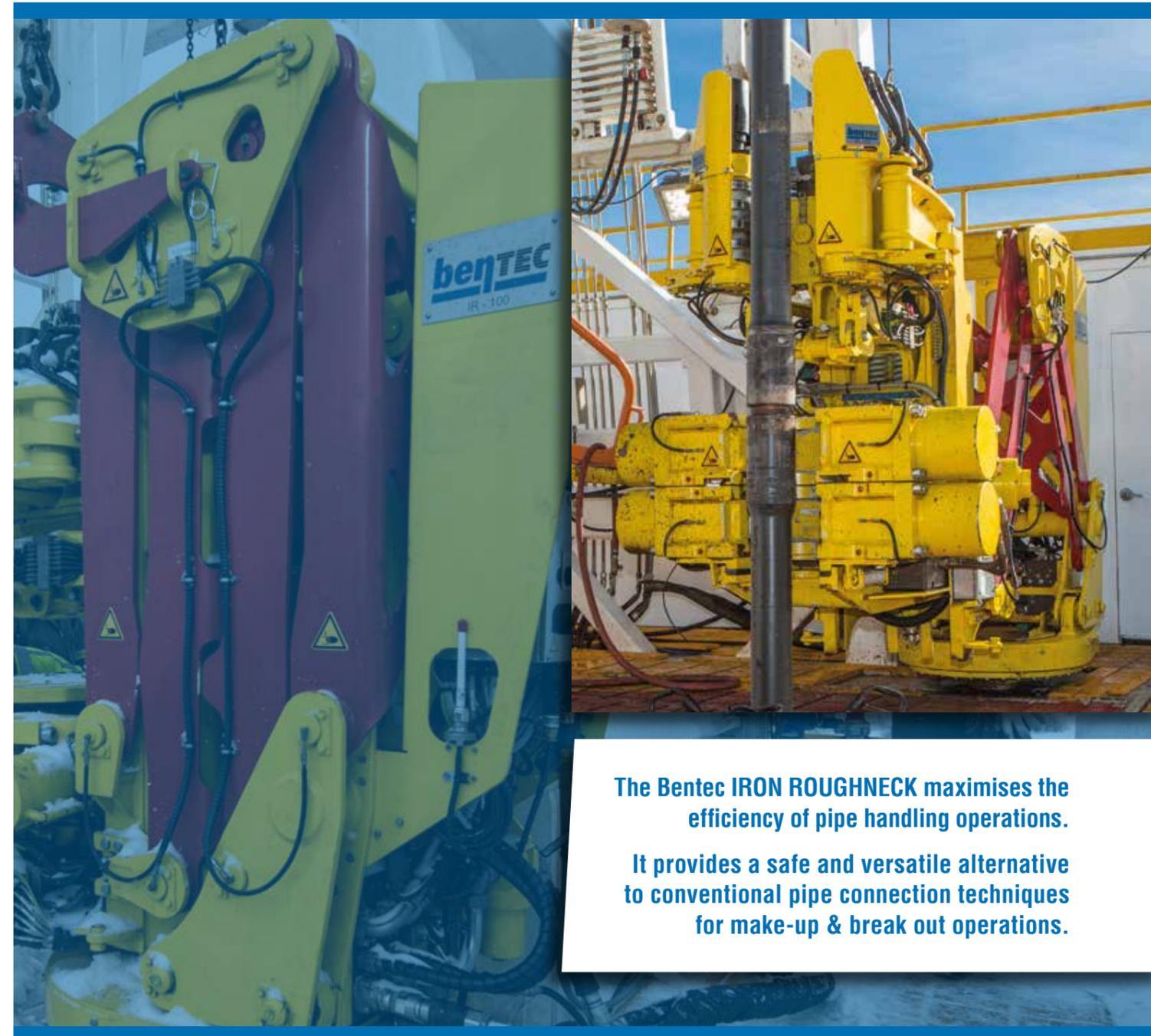
The Bentec IRON ROUGHNECK maximises the efficiency of pipe handling operations.
