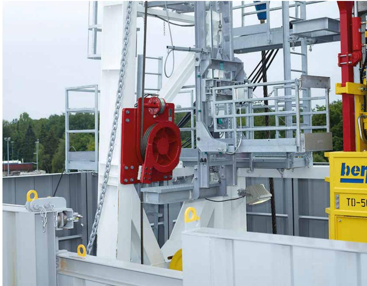
Designed for use with compression load cells, Bentec Deadline Anchors are made from high-grade structural steel for operations in the harshest environments, from -40°C up to +55°C.
