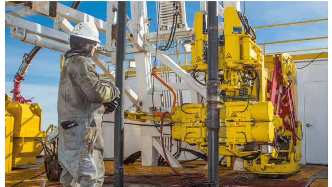
Over the past 40 years, Bentec has developed an impressive portfolio of automated tubular running operations in order to build more robust and reliable Iron Roughnecks that reduce both downtime and maintenance. The Iron Roughneck is available in two versions.
